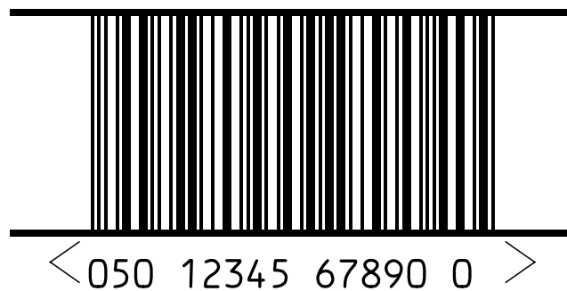
ITF-14 barcode with X-dimension of 0.495 mm
